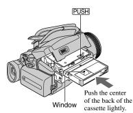
The cassette compartment automatically slides back in. Do not force the cassette into the compartment. This may cause a malfunction.
