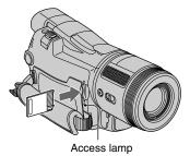
If you force the "Memory Stick Duo" into the slot in the wrong direction, the "Memory Stick Duo," the "Memory Stick Duo" slot, or image data may be damaged.
