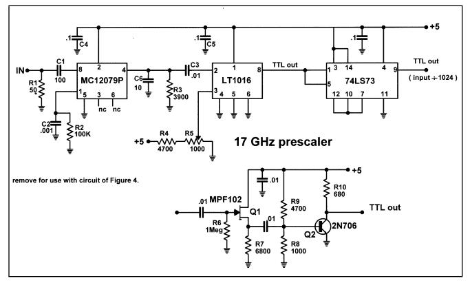
Figure 2. Prescaler built around a MC12079.
