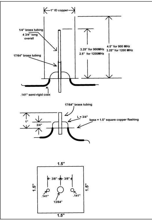
Figure 7. Coaxial filters.
