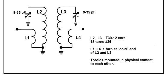
Figure 1. Double-tuned circuit.
