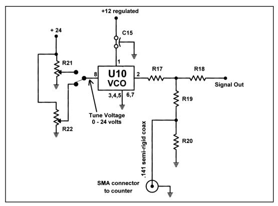
Figure 4. Simple generator capable of 940-2300 MHz.
