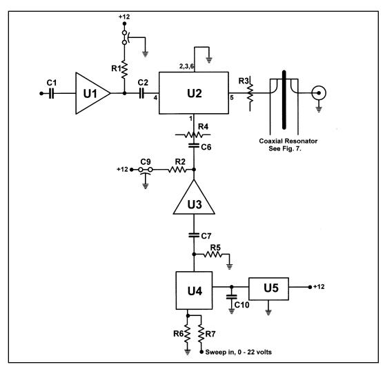
Figure 5. Method for reaching higher frequencies.
